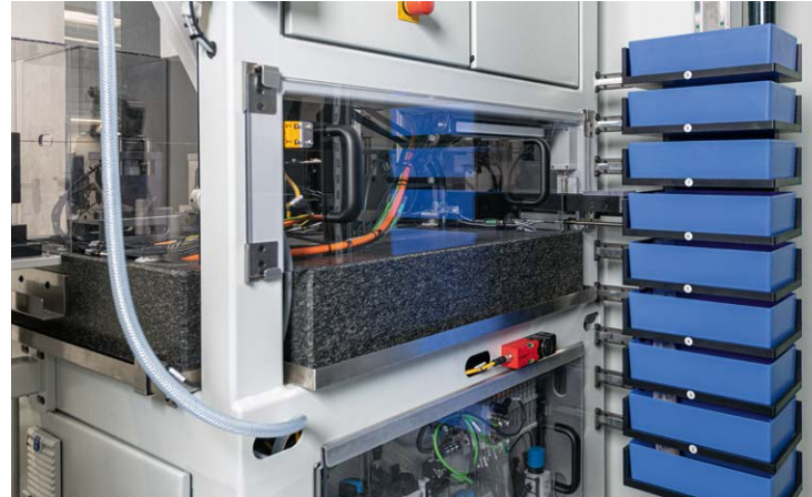
Separator for the collection of finished workpieces.
