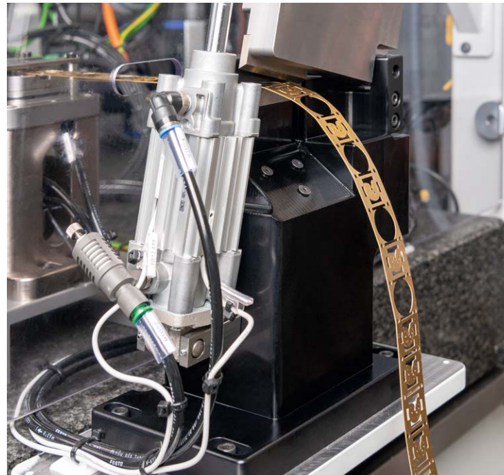
Separator for the collection of finished workpieces.
