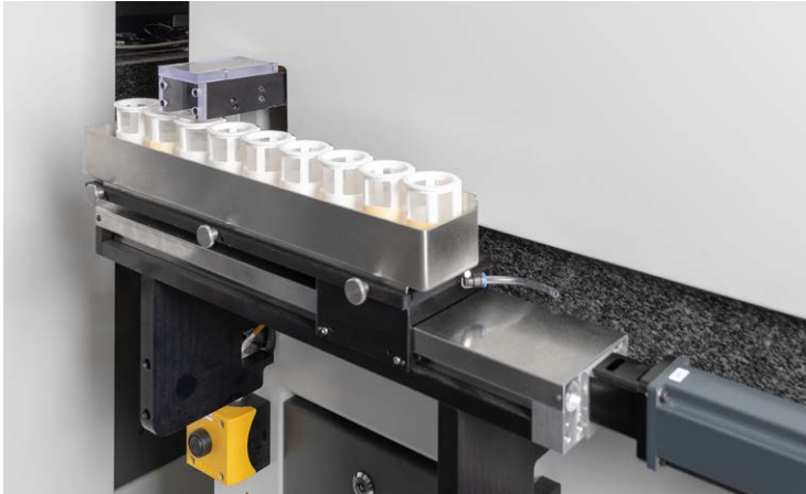
Separator for the collection of test parts.
